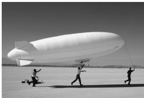
Fig. 3 NASA JPL Titan Aerobot Testbed
